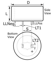
General InformationSeriesFGDescriptionRadial Cylindrical Double Layer CapacitorRoHSYesAEC-Q200NoComponent Weight5.2 gMiscellaneousDischargeValue = 2.2 F.
