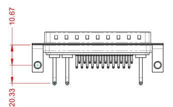
10A (CURRENT) POWER/CO-AX CONTACT RATING: (IF PRESENT) SIGNAL CONTACT CURRENT RATING: 5A PER CONTACT SIGNAL CONTACT RESISTANCE:  $10m\Omega$  MAX. **INSULATOR RESISTANCE:** 5000MΩ min. DIELECTRIC
