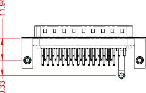
30A (CURRENT) POWER/CO-AX CONTACT RATING: (IF PRESENT) SIGNAL CONTACT CURRENT RATING: 5A PER CONTACT SIGNAL CONTACT RESISTANCE:  $10m\Omega$  MAX. **INSULATOR RESISTANCE:** 5000MΩ min.
