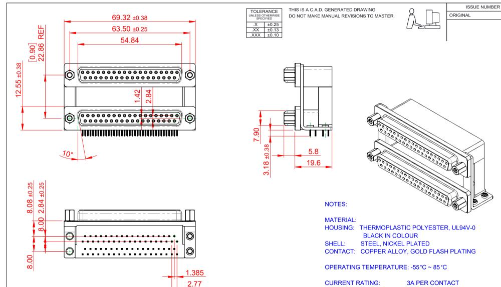
CURRENT RATING:3A PER CONTACTCONTACT RESISTANCE:25mΩ MAX.INSULATOR RESISTANCE:5000MΩ min.DIELECTRICWITHSTANDING VOLTAGE:100V AC rms
