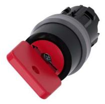
Key-operated switch O.M.R, 22 mm, round, plastic with metal front ring, lock number 73037, red, with 2 keys, 2 switch positions O<I, momentary contact type, Actuating angle 45°, 10:30h/12h, key removal O, with laser labeling, upper case and lower case, always upper case at the beginning of the word
