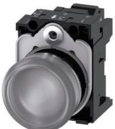
Indicator lights, 22 mm, round, metal, shiny, clear, lens, smooth, with holder, LED module with integrated LED 24 V AC/DC, spring-type terminal, with laser labeling, upper case and lower case, always upper case at the beginning of the word
