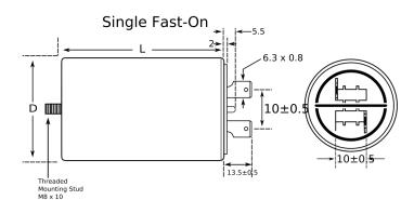
Series C27 Dielectric Film/Foil Polypropylene Style Plastic Case and Cover, Ultra Sonically Welded Description Ultra Sonically Welded Seal, Safety Class PO, Features UL 94 V0 Disk **RoHS** Yes Lead Fast On (1+1) UL, VDE, UL (Construction Only), UL\_94 VO Qualifications Disk AEC-Q200 No Component 26 g Weight
