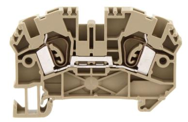
Feed-through terminal, Tension-spring connection, Mounting type: Mounting rail TS 35/7.5, Rated cross-section: 4 mm<sup>2</sup>, Width: 6.1 mm, Colour: Beige
