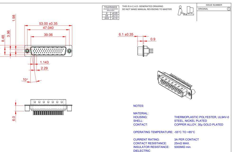
WITHSTANDING VOLTAGE: 1000V AC rms
