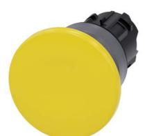
Mushroom pushbutton, 22 mm, round, plastic with metal front ring, yellow, 40mm, momentary contact type, with laser labeling, symbol number according to, ISO 7000 or IEC 60417
