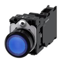
Illuminated pushbutton, 22 mm, round, plastic, blue, pushbutton, flat, momentary contact type, with holder, 1 NO+1 NC, LED module with integrated LED 24 V AC/DC, spring-type terminal, with laser labeling, upper case and lower case, Always upper case at the beginning of the word
