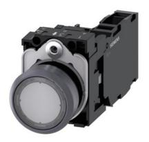
Illuminated pushbutton, 22 mm, round, plastic with metal front ring, clear, pushbutton, flat, momentary contact type, with holder, 1 NO+1 NC, LED module with integrated LED 24 V AC/DC, screw terminal, with laser labeling, upper case and lower case, Always upper case at the beginning of the word
