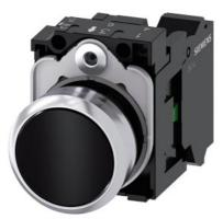
Pushbutton, 22 mm, round, metal, shiny, black, pushbutton, flat, momentary contact type, 1 NO, spring-type terminal, Z=20-unit packaging
