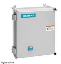
Reversing motor starter, Size 2 1/2, Three phase full voltage, Amb. compensate bimetal OLR, Contactor amp rating 60A, 24VAC 50-60Hz coil, Non-combination type, Enclosure type 4X fiberglass, Water/dust tight noncorrosive
