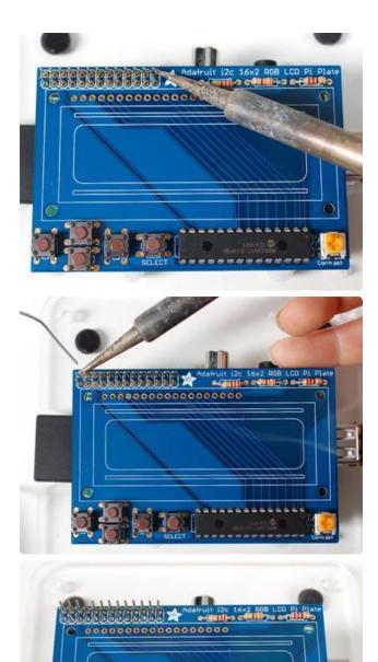
Now we will solder all 26 pins for the plate - this will send power and data between the two boards and also provide a mechanical stability. You may need to hold the plate down with tape to get it sitting flat against the Pi.
