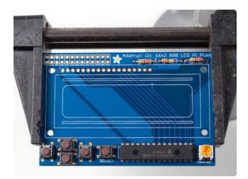
We're nearly done! Now we will place the I2C port expander chip. Double check that it has the MCP23017-E/SP marking on it. This is a 16-pin expander chip, that uses the i2c bus. That means you can send it commands using the i2c pins on an Pi and control 16 more digital pins! 5 of those pins go to the buttons, 6 go to the LCD control and 3 are used for the backlight (the remaining 2 are unused).
