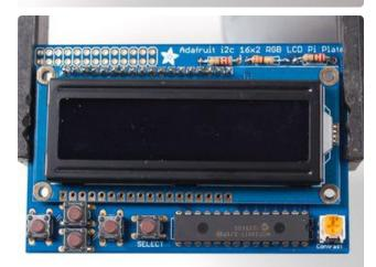
Slide the LCD over the header so that it is perfectly centered over the four holes and the silkscreen.
