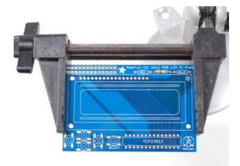
Put the printed circuit board into a vise or board holder, heat up your soldering iron and make sure you're ready to go! We'll start with the first resistor GREEN which has orange, orange, brown, gold bands on it. This resistor acts as the backlight control resistor for the green backlight pin.
