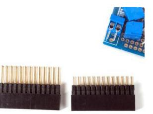
Next we will attach the header, there is a standard 'extra tall' header included in the kit. However, if you want to attach a cobbler or GertBoard, etc to the plate, you may want to opt for one of our stacking headers, they're extra long so you can plug in an IDC cable on top!
