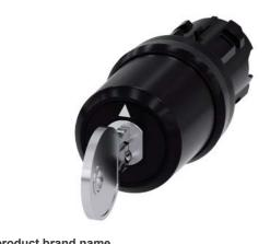
Key-operated switch BKS, 22 mm, round, plastic, lock number S1, with 2 keys, 3 switch positions I-O-II, latching, actuating angle 2x45°, 10:30h/12h/13:30h, key removal I, with laser labeling, upper case and lower case, always upper case at beginning of line
