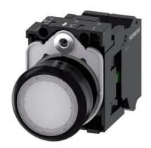
Illuminated pushbutton, 22 mm, round, plastic, white, pushbutton, flat, momentary contact type, with holder, 1NO, LED module with integrated LED 24 V AC/DC, spring-type terminal, with laser labeling, upper case and lower case, always upper case at beginning of line
