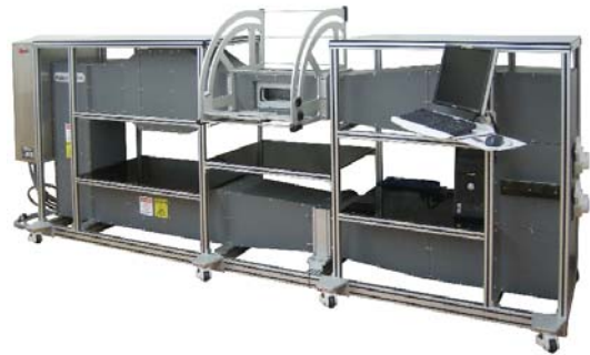
Fig. F: FDK Original Wind Tunnel
