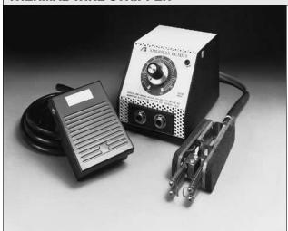
The ease and simplicity of operation of the Thermal Wire Stripper make it ideal for most strain gage leadwire stripping. The variable heat control allows stripping of all thermoplastic insulations, including Teflon®, in sizes No. 18 to No. 36 AWG (1 to 0.1 mm diameter). The foot switch and tweezer hand- piece give excellent operator control over the stripping operation. Includes power unit and foot switch, both with 3-wire NEMA plugs, and tweezer handpiece.
