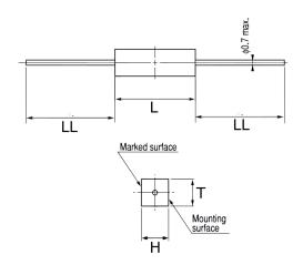
**General Information** Series OHD Thermal Reed Switch Type Style Axial Description Thermal Guard High Reliability, High-Speed Response, Long Features Operational Life, Excellent Environmental Durability, High Temperature Accuracy Lead Wire Leads RoHS Yes REACH Yes Qualifications UL, CSA, TUV
