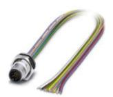
Sensor/actuator flush-type plug, 17-pos., M12 SPEEDCON, rear/screw mounting with M16 thread, with 0.5 m halogen-free TPE litz wire,  $17 \times 0.14 \text{ mm}^2$
