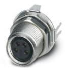
Sensor/actuator flush-type connector, socket, 4-pos. M8, rear/screw mounting with M10 fastening thread, with straight solder connection
