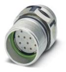
Device connector for front wall, straight, shielded: yes, for standard and SPEEDCON interlock, M23, No. of pos.: 12, type of contact: Socket, Crimp connection, Axial seal, Central fastening M20 x 1.5, can be positioned via a locking nut
