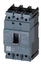
circuit breaker 3VA5 UL frame 125 breaking capacity class S 25kA @ 480 V 3-pole, line protection TM210, FTFM, In=15A overload protection Ir=15A fixed short-circuit protection Ii=20 x In nut keeper kit on both sides
