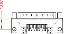
**OPERATING TEMPERATURE:** -55°C ~ 125°C 75Ω (IMPEDANCE) POWER/CO-AX CONTACT RATING: (IF PRESENT) SIGNAL CONTACT CURRENT RATING: 5A PER CONTACT SIGNAL CONTACT RESISTANCE:  $10m\Omega$  MAX. INSULATOR RESISTANCE:
