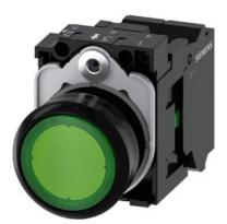
Illuminated pushbutton, 22 mm, round, plastic, green, pushbutton, flat, momentary contact type, with holder, 1NO, LED module with integrated LED 110 V AC, spring-type terminal, with laser labeling, upper case and lower case, Always upper case at the beginning of the word
