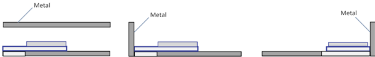
Fig 5-4. Not recommended location in Z plane
