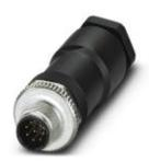
Connector, 8-position, Plug straight M12, A-coded, Screw connection, knurl material: Zinc die-cast, nickel-plated, cable gland Pg11, external cable diameter 8 mm ... 10 mm
