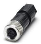
Connector, 5-position, Socket straight M12, A-coded, Spring-cage connection, knurl material: Zinc die-cast, nickel-plated, external cable diameter 4 mm  $\dots$  8 mm
