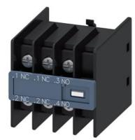
Auxiliary switch on the front, 1 NO + 2 NC Current path 1 NC, 1 NC, 1 NO for 3RH and 3RT Ring cable lug connection .1/.2, .1/.2, .3/.4
