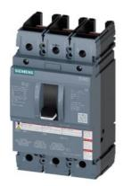
molded case switch 3VA5 UL frame 250 max. sh-circ breaking capacity 100kA @ 480V 3-pole, line protection MCS110, In=150A without overload protection self-protection li=16 x In without connection
