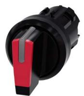
Selector switch, illuminable, 22 mm, round, plastic, red, selector switch, short, 3 switch positions I-O<II, left latching, right momentary contact type, actuating angle  $2x45^{\circ}$ , 10:30h/12h/13:30h, with laser labeling, upper case
