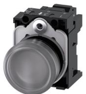
Indicator lights, 22 mm, round, plastic, clear, lens, smooth, with holder, LED module, with integrated LED 24 V AC/DC, spring-type terminal, Z=20-unit packaging
