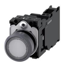
Illuminated pushbutton, 22 mm, round, plastic with metal front ring, clear, pushbutton, flat, momentary contact type, with holder, 1 NO+1 NC, LED module with integrated LED 24 V AC/DC, spring-type terminal, with laser labeling, symbol number according to, ISO 7000 or IEC 60417
