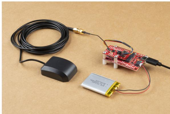
*This demo circuit uses the SparkFun GPS Breakout - ZOE-M8Q (Qwiic) and GPS/GNSS Magnetic Mount Antenna.*
