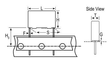
Series F872 Dielectric Metallized Polypropylene Style Radial Features MKP EMI Safety RoHS Yes Lead Wire Leads Safety Class X1 Qualifications ENEC, UL, cUL, CQC AEC-Q200 No THB Performance No 12.09 g Component Weight Miscellaneous ClimCat: 40/110/56/B Shelf Life 104 Weeks
