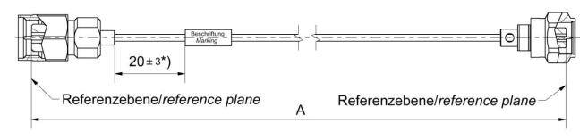
All dimensions are in mm; tolerances:  $\pm$  3mm for A  $\leq$  300 mm;  $\pm$  1% for A > 300 mm\*) If length "A"  $\leq$  90 mm marking is mount centric  $\pm$  5mm
