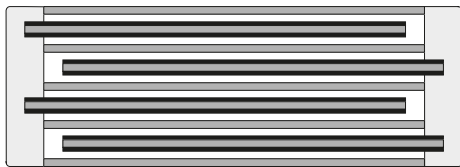
Extended double side metallized carrier film design
