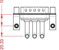
40A (CURRENT) POWER/CO-AX CONTACT RATING: (IF PRESENT) SIGNAL CONTACT CURRENT RATING: 5A PER CONTACT SIGNAL CONTACT RESISTANCE:  $10m\Omega$  MAX.
