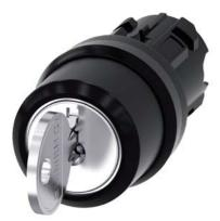
RONIS key-operated switch, 22 mm, round, plastic, lock number SB30, with 2 keys, 3 switch positions I-O<II, left latching, right momentary contact type, actuating angle 2x45°, 10:30h/12h/13:30h, key removal O+I, possible special locks: SB31, 421, 455, with laser labeling, inscription or symbol Customer-specific selection with SIRIUS ACT configurator (CIN)
