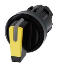
Selector switch, illuminable, 22 mm, round, plastic, yellow, selector switch, short, 3 switch positions I-O<II, left latching, right momentary contact type, actuating angle  $2x45^{\circ}$ , 10:30h/12h/13:30h, with laser labeling, upper case and lower case, always upper case at the beginning of the word
