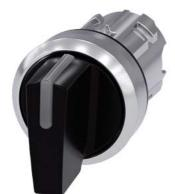
Illuminable selector switch, 22 mm, round, metal shiny, black, Selector switch short, 3 switch positions I>O<II, momentary contact type, actuating angle  $2x45^{\circ}$ , 10:30 /12 /13:30, Z=50-unit packaging
