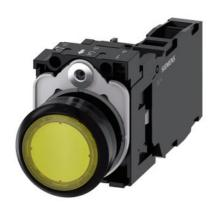
Illuminated pushbutton, 22 mm, round, plastic, yellow, pushbutton, flat, momentary contact type, with holder, 1 NO+1 NC, LED module with integrated LED 24 V AC/DC, screw terminal, with laser labeling, lower case
