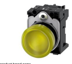
Indicator lights, 22 mm, round, Metal, shiny, yellow, lens, smooth, with holder, LED module with integrated LED 230 V AC, screw terminal, with laser labeling, upper case
