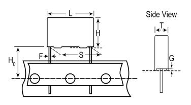
General Information Series F881 Dielectric Metallized Polypropylene Style Radial Features MKP, Pulse RoHS Yes Wire Leads Lead Safety Class Qualifications ENEC, UL, cUL, CQC AEC-Q200 No THB Performance No 7.075 g Component Weight Miscellaneous ClimCat: 40/110/56/B Shelf Life 104 Weeks
