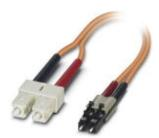
Assembled FO cable, zip cord cable, multi-mode fiberglass 50/125  $\mu$ m, OM2, plug: LC/SC duplex, degree of protection: IP20, for installation in cable ducts or control cabinets, length: 2 m
