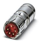
Cable connector, straight long, shielded: yes, SPEEDCON locking, M40, No. of pos.: 8+4+PE, type of contact: Pin, Crimp connection, cable diameter range: 14 mm ... 20.5 mm
