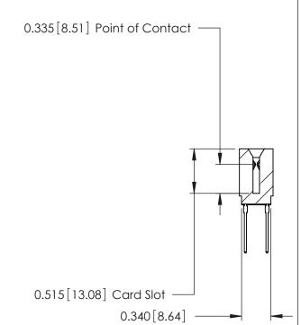
ACAD REFERENCE NO. 746-ENG MASTER 746 Series Ultra-Mate Card Edge Connector - Press Fit DRAWN: J.LEE DATE: AUG 20/09 Part Number: 746-046-545-201 CHECKED: DATE: **EDAC INC** SCALE: SHEET 1 OF 1 THESE DRAWINGS AND SPECIFICATIONS ARE THE PROPERTY OF EDAC INC.,AND TORONTO, ONTARIO SHALL NOT BE REPRODUCED, OR COPIED DRAWING NUMBER CANADA OR USED AS THE BASIS FOR THE 746-ENG MASTER MANUFACTURE OR SALE OF APPARATUS YOUR CONNECTION TO QUALITY & SERVICE WITHOUT WRITTEN PERMISSION.
