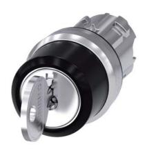
RONIS key-operated switch, 22 mm, round, metal, shiny, lock number SB30, with 2 keys, 3 switch positions I-O<II, left latching, right momentary contact type, actuating angle 2x45°, 10:30h/12h/13:30h, key removal O, possible special locks: SB31, 421, 455, with laser labeling, upper case and lower case, always upper case at beginning of line
