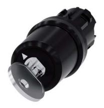
key-operated switch Siemens, 22 mm, round, plastic, lock number SSG10, with 2 keys, 2 switch positions O-I, latching, actuating angle  $90^\circ, 10:30h/13:30h,$  key removal O+I, with laser labeling, lower case
